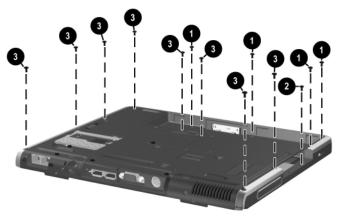
Removing the Top Cover Screws
